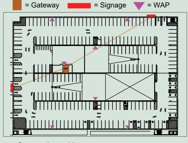
Gateway located in secure area RS-485 connection from gateway to signage Wireless access points installed for complete coverage (locations garage dependent)
